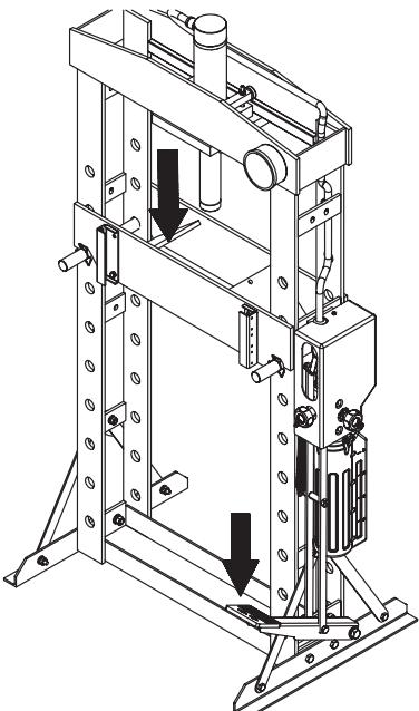
5. Turn the Release Valve and Fast-slow Valve counterclockwise.
