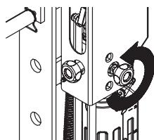
8. Align ram and workpiece to ensure center-loading, pump the handle or pedal. Do not overload workpiece.
