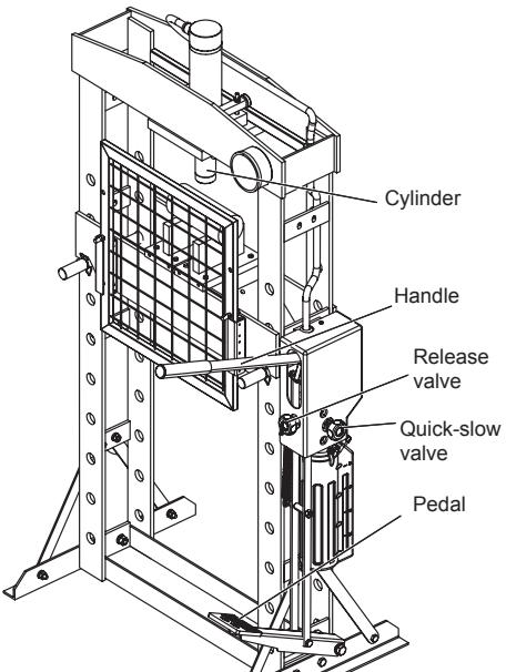
5. Close the release and Fast-slow Valve valve by turning it clockwise until it is firmly closed.
