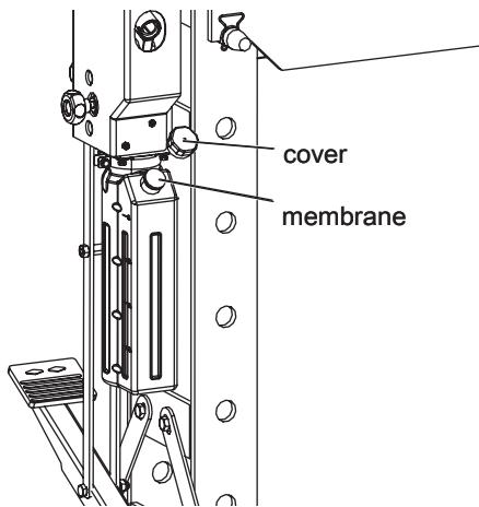
4. Turn the jack on its side so that old oil will drain from the oil fill hole.
