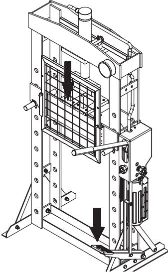
9. When work is completed, stop pumping the handle. Slowly turn the release valve counter-clockwise in small increments until ram is free from work piece.
