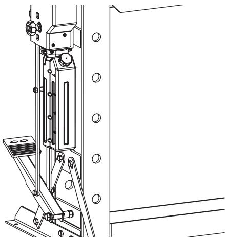
3. Fill the oil case until oil level is near the 1.8L of the oil tub.
