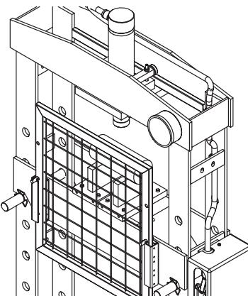
2. Place bolster plates (18) on press bed frame. Place work piece on the bed frame or pressing block, use every precaution necessary to ensure safety and to prevent accidents. Position work piece in a manner which will not allow it to inadvertently fall from the bed frame or pressing block.
