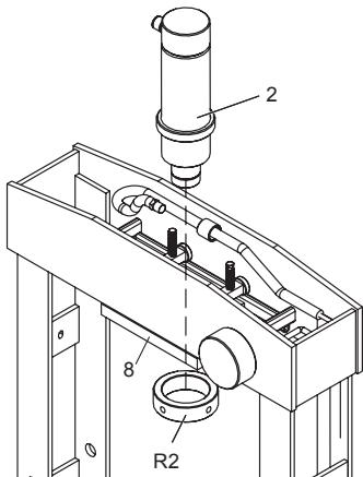
7. Connect the male coupling hose connector (45) to cylinder assembly (2).
