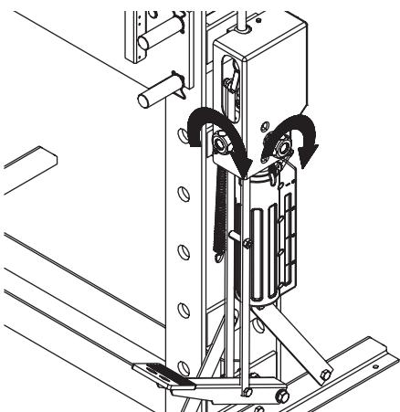
4. Step on the pedal to extend the piston rod for a few distance.
