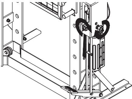
6. Pump the handle or pedal until serrated saddle nears workpiece. Then, open Fast-slow Valve by turning it counterclockwise.
