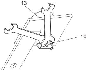
5. Locate the hydraulic hose fitting on the hose assembly (45). Install the O-ring (9) into the groove of the hose connection fitting (45). Then Connect the hydraulic hose (45) to the gauge (13). Securely tighten the hose fitting (45) on the gauge (13).
